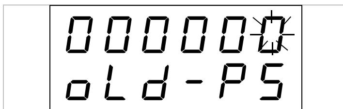
If inputted is Operator Password, this operation interface will be skipped; if inputted is Administrator Password, ‘Administrator Password [AP]’ or ‘Operation Password [oP]’ can be modified via **【▶】** **【▲】**.
