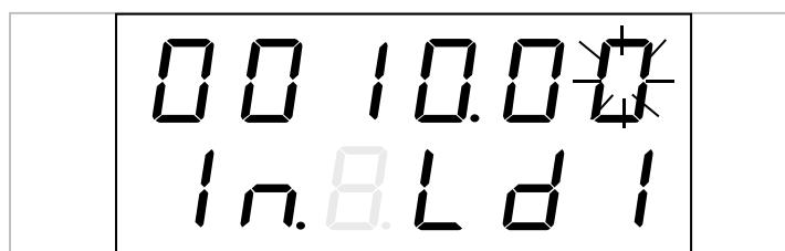
Loading 'Correction Point's Loading Weight 1' on the weigher,
